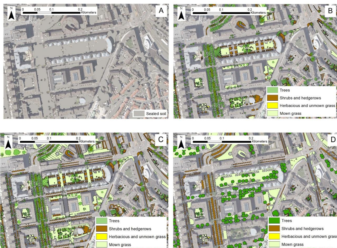
Figure 5. Greenspace design per scenario in example area 1. A: Scenario 'No greenspace'. B: Scenario 'Current greenspace'. C: Scenario 'Green parking lots and squares'. D: Scenario 'Optimized greenspace locations'.
