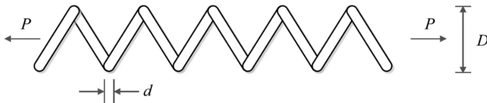
Figure 12. Schematic of the tension/compression spring design.
