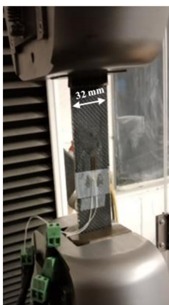
Figure 7. Tensile test performed on a coupon instrumented with strain gages using an Instron® 3382 universal testing system.
