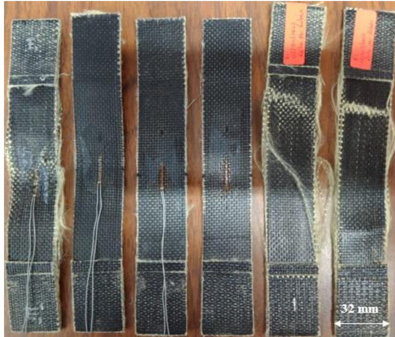
Figure 11. Condition of coupons after the tensile test at 0^\circ .
