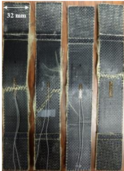
Figure 13. Condition of coupons after the tensile tests at 90°.
