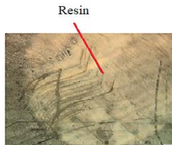
Figure 3. Resin film over brake pad analysis area.
