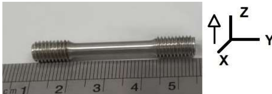
Figure 1. Machined tensile sample based on ASTM E8 standard with its longitudinal axis aligned with the Y direction, perpendicular to the building Z-LPBF direction .
