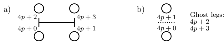
Figure 14. Assignment of leg numbers to operator legs for an operator at propagation step p . a) Illustration of a two-site operator with four real vertex legs. b) Illustration of a single-site operator with only two real vertex legs and two ghost legs.
