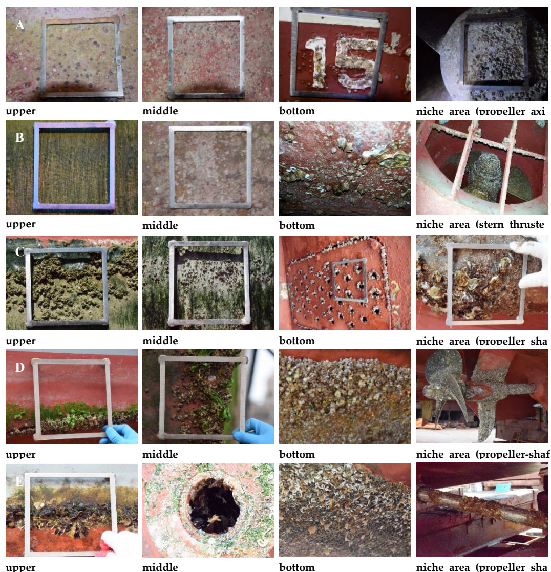
Figure 3. Attached hull-fouling macroinvertebrates on the five research vessels ((A): Isabu, (B): Onnuri, (C): Eardo, (D): Jangmok 1, (E): Jangmok 2; upper: waterline on the hull side, middle: between the waterline and bottom line, bottom: including the seawater inlet, niche areas: propeller, shaft, and thruster; quadrats: 15x15 cm).
