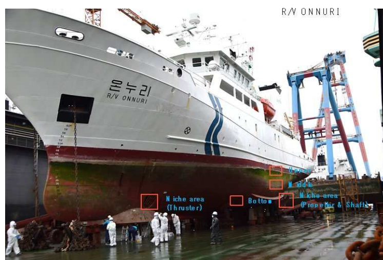
Figure 1. Sampling locations for attached hull-fouling macroinvertebrates. Samples were collected 3–5 times repeatedly using quadrats (15 x 15 cm) in each sector: upper, middle, bottom, and niche areas (propeller shaft or thruster).
