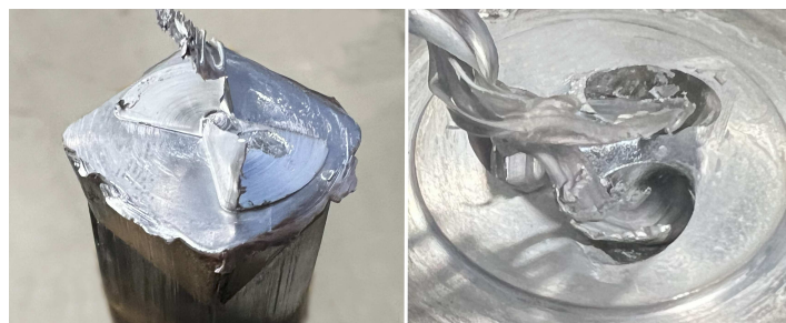
Figure 6. Ribbon formation (extrudate) as generated by two different die designs: bow-tie # 1 (left, end of rod with visible bulging) and 45° tri-hole # 4 (right, still within die).
