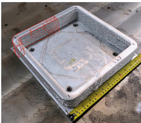
Figure 11. Completed sample component with base plate after the deposition process. Tensile specimens were extracted from the positions indicated in red.
