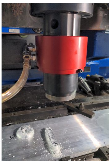
Figure 4. Tool-holder with cooling collar (red), mounted die (silver) and fixturing. Background: linear and doughnut shaped test extrusions.
