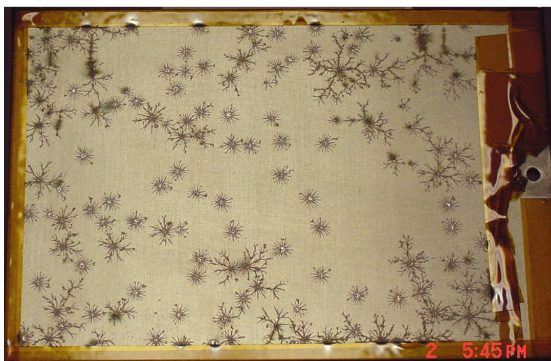
Figure 1. Anodized aluminium breakdown in a plasma environment [40]
