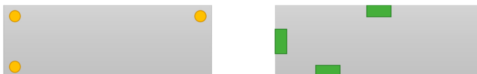
Figure 7. Optimal placement obtained from the Effective Independence (EI) for 3 accelerometers (left) and 3 PVDFs (right) (adapted from [42]).
