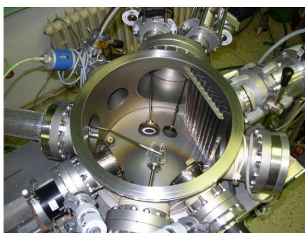
Figure 13. a) Scheme of dual PLD using two lasers and two targets, b) photo of the deposition chamber, c) photo of the deposition process.
