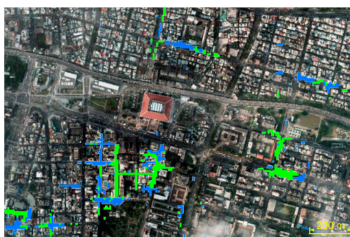
Figure 2. Part of the flood hazard map of Taipei City, Taiwan under short duration, high intensity rainfall. The colored area represents the inundation zone.
