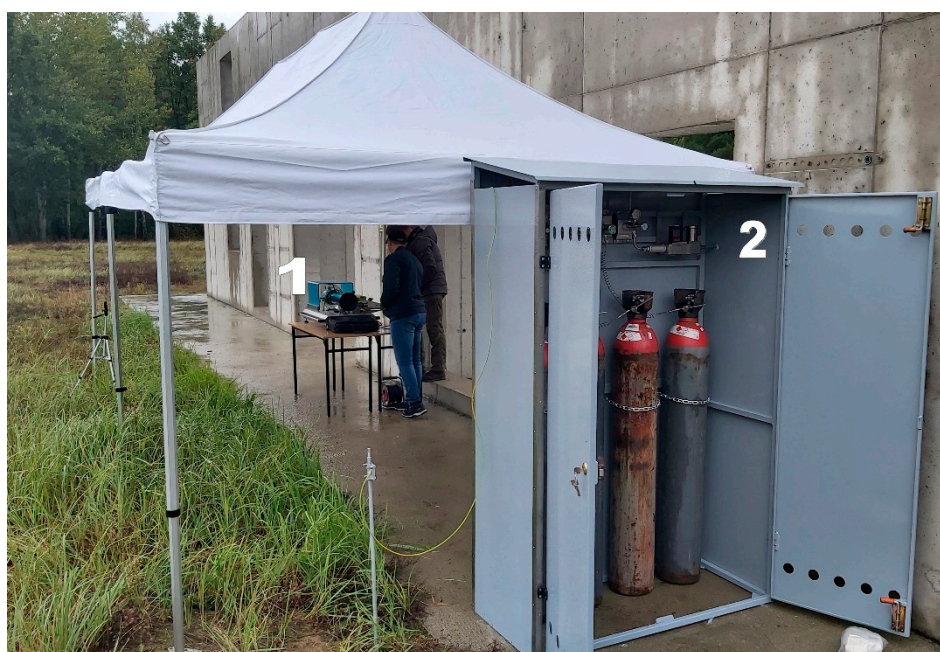
Figure 2. Place of research: 1 - engine test stand, 2 - hydrogen connection station.
