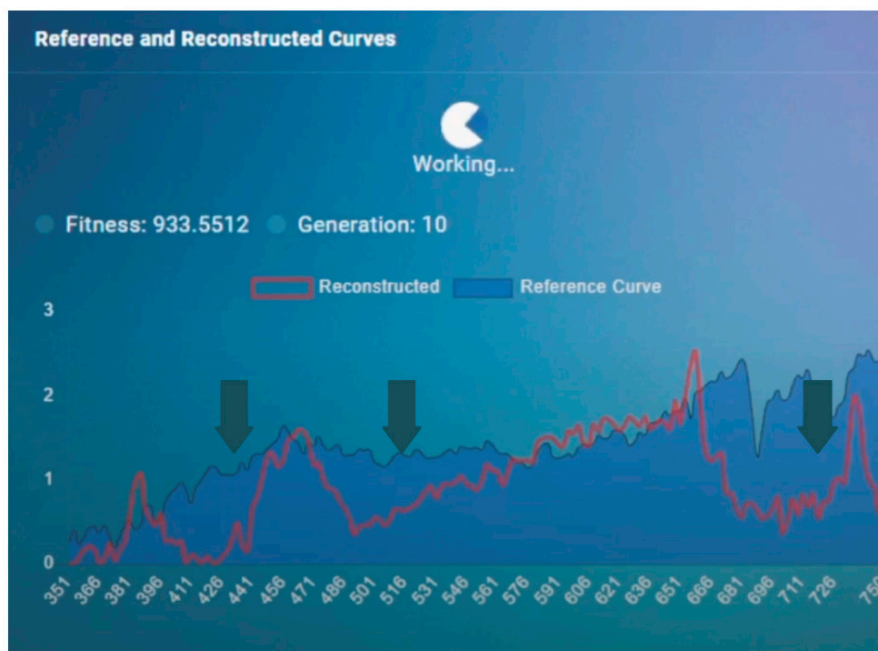
Figure 3. Example of one generated curve and its relation to the measured HOCR curve with missing LEDs covering the areas around 426, 516 and 726 nm.
