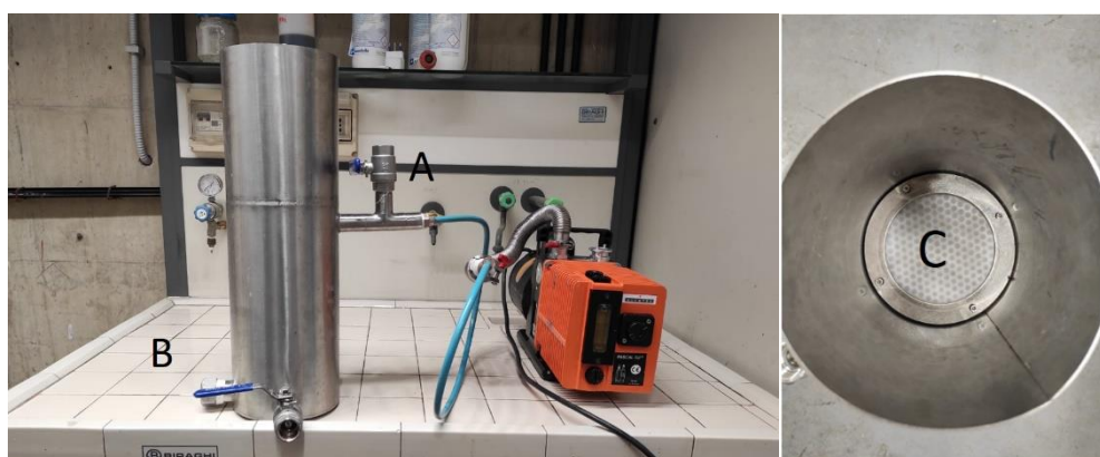
Figure 1. Experimental filter for the removal of suspended solids from vegetation water: (A) Hydraulic valve connecting the lower chamber with a vacuum pump; (B) filtered water drain valve; (C) top vision of the filter with the support technical sheet.
