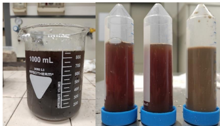
Figure 5. The left picture shows samples S120, S500 and US collected for COD measurement; in the right picture vegetation water filtered and neutralized at pH 5.5.
