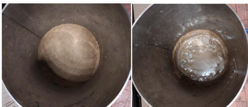
Figure 4. Clean straw filter (left picture); solid residues on the filter surface (right picture).
