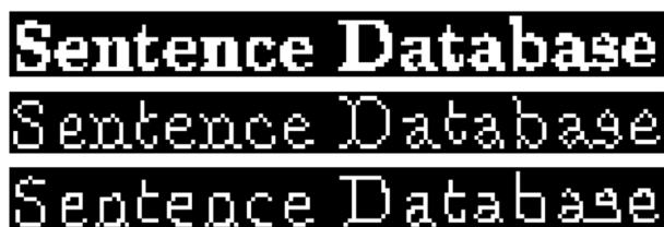
Figure 1. S/T Algorithm Illustration - Input Text (top); Zhang-Suen (middle); Guo-Hall (bottom) - Originally from [10].
