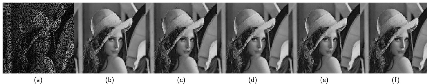
Figure 6. Sparse reconstruction results for blocked DCT scenario: (a) CSed image ( M = 0.4 ); (b) reconstructed by the TwIST (MSE = 191.46); (c) reconstructed by the SALSA (MSE = 273.30); (d) reconstructed by the NESTA (MSE = 181.81); (e) reconstructed by the YALL1 (MSE = 189.69); (f) reconstructed by the FICI-TwIST (MSE = 176.99).
