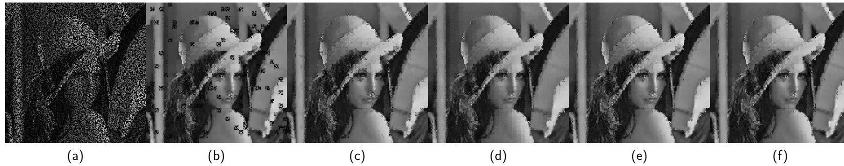
Figure 8. Sparse reconstruction results for blocked DWT scenario: (a) CSed image ( M = 0.4 ); (b) reconstructed by the TwIST (MSE = 1093.89); (c) reconstructed by the SALSA (MSE = 527.58); (d) reconstructed by the NESTA (MSE = 447.90); (e) reconstructed by the YALL1 (MSE = 481.04); (f) reconstructed by the FICI-TwIST (MSE = 432.41).
