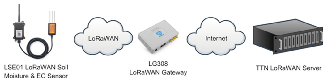
Figure 2. LoRaWAN used for continuous soil moisture data collection [28].
