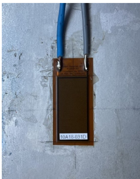
Figure 12. Piezoelectric patch directly bonded to the plate.
