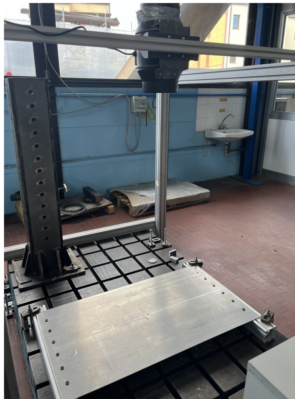
Figure 10. Clamped plate and fan for the excitation of the plate through the air jet.
