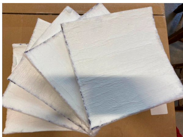
Figure 2. The aerogel-enhanced blanket.
