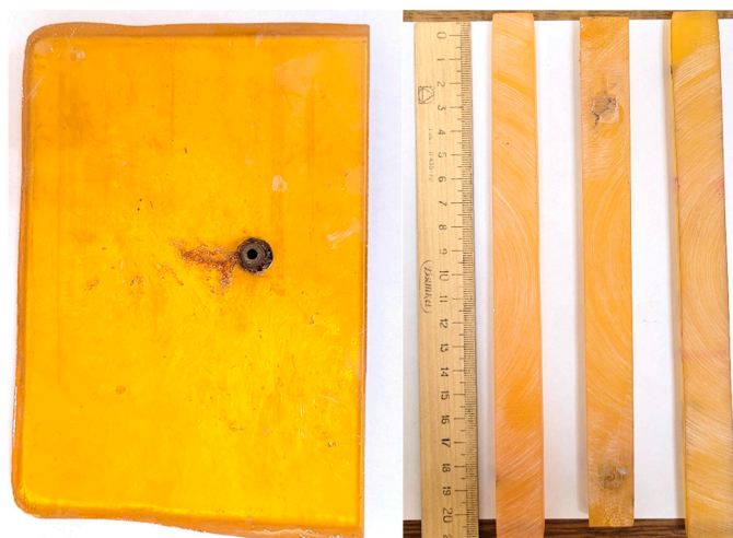
Figure 1. Epoxy plate and cut out rod samples after machining.
