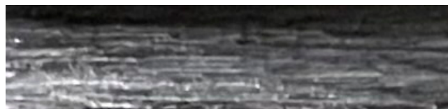
Figure 19a. The state of the tooth surface for single hobbing with the axial feed of 1mm/r.
