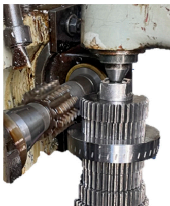
Figure 16. The diagram of the gear blank after the cutter aligning.
