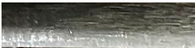
Figure 19b. The state of the tooth surface for single hobbing with the axial feed of 0.5mm/r.
