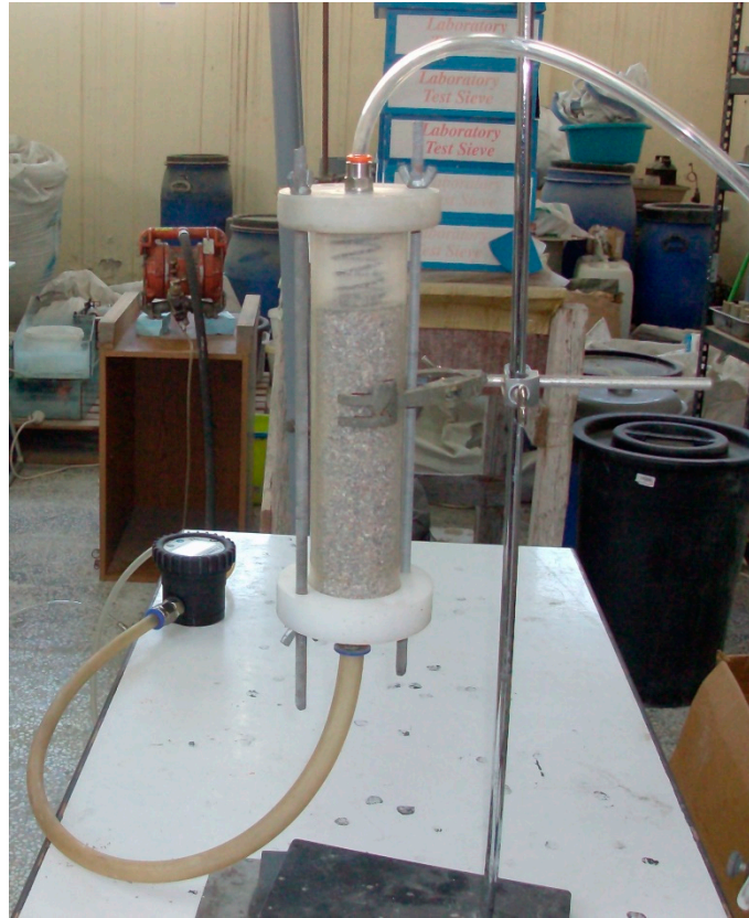
Figure 6. Set-up for determination of permeability coefficient of pure sands.
