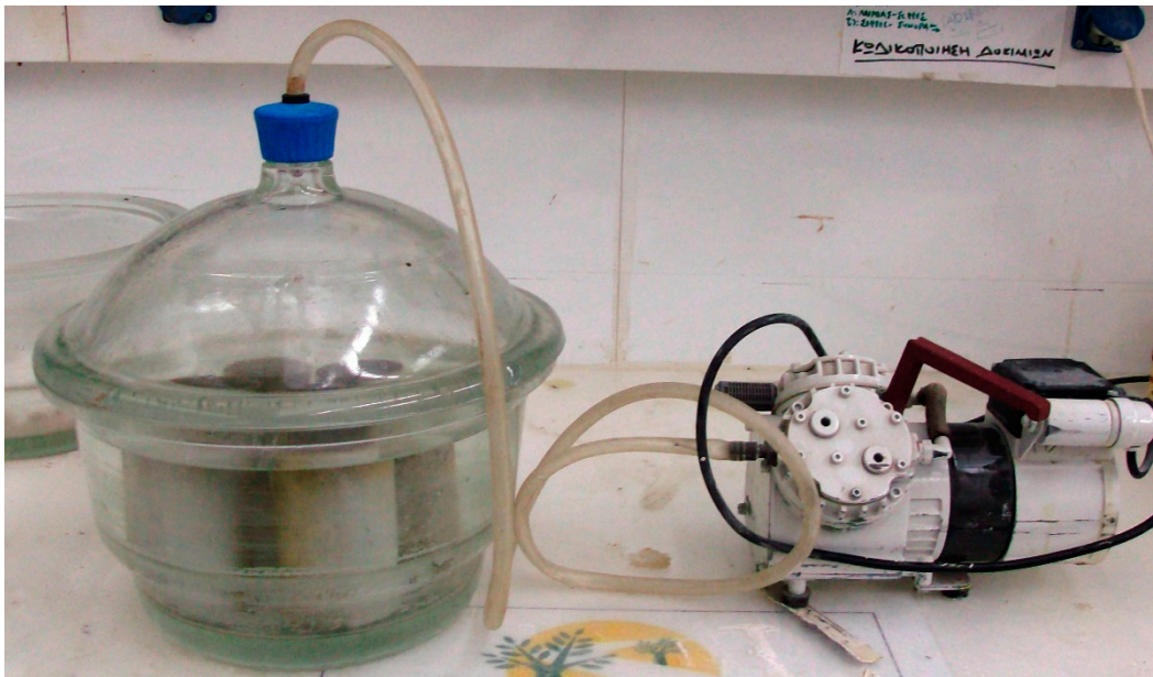
Figure 5. Vacuum saturation device for porosity measurements of grouted sands.
