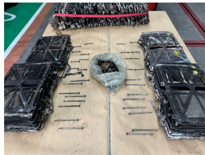
Figure 7. Burnt Nissan Leaf battery disassembled in the arrangement in which it is in the vehicle.
