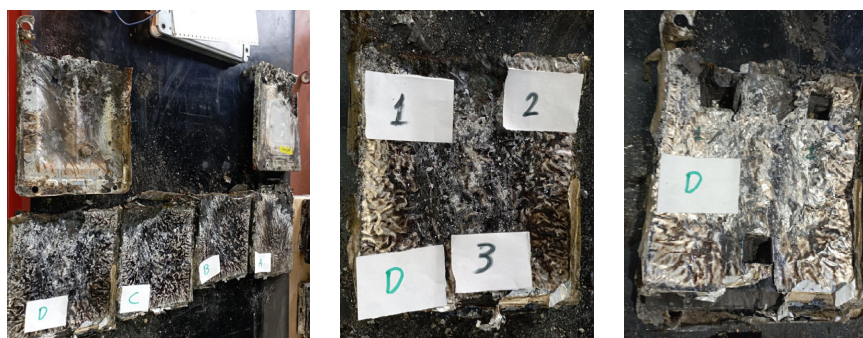
Figure 13. Obtaining samples from a module 30 calcined cell.
