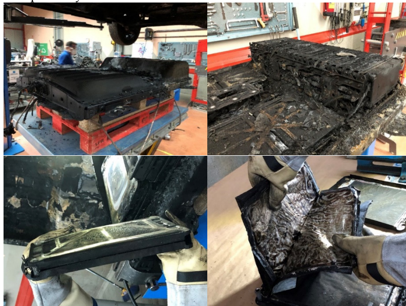
Figure 5. Pictures of the state of the battery pack, the module, and the lithium-ion cells inside the battery pack.
