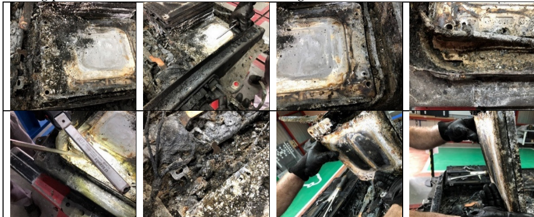
Figure 8. Images of the condition of module 30 (horizontal arrangement) of the battery pack of the burnt Nissan Leaf vehicle. This module has been identified as the most damaged between the modules in the horizontal arrangement.
