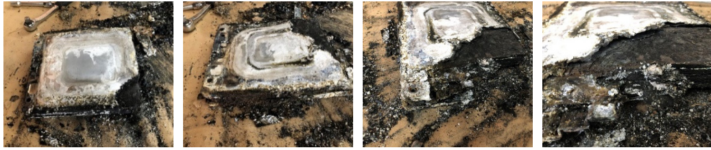
Figure 9. Images of the condition of module 11 (vertical arrangement) of the battery pack of the burnt Nissan Leaf vehicle. This module has been identified as the most damaged between the vertically arranged modules.
