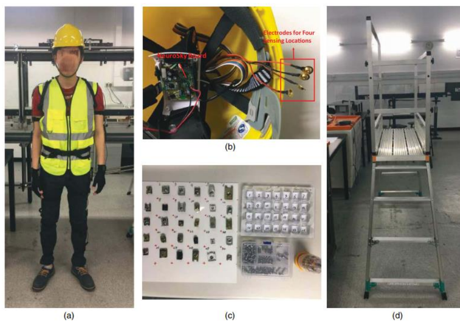
Figure 4. Experimental apparatus: (a) experiment subject; (b) EEG hardhat and the EEG monitoring chips; (c) nuts and bolts; (d) ladder platform [51].
