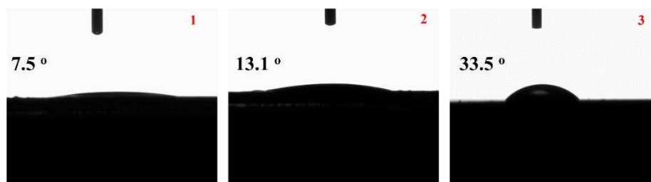
Figure 2. Images of water contact angles of (1) MC, (2) MCC and (3) NC samples.
