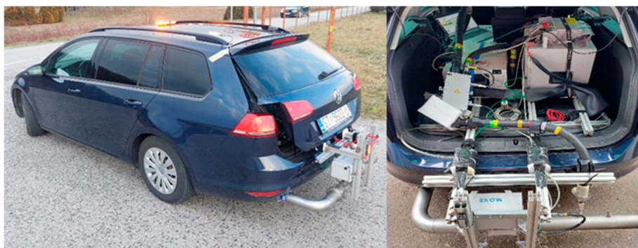
Figure 2. Test vehicle with built-in measuring equipment.
