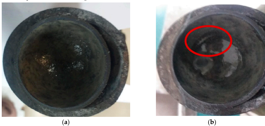
Figure 6. Acetabular implant with double Sol-gel/porcelain layer: (a) after the coating deposition and before wear test; (b) after the simulation wear test for 100,000 cycles.
