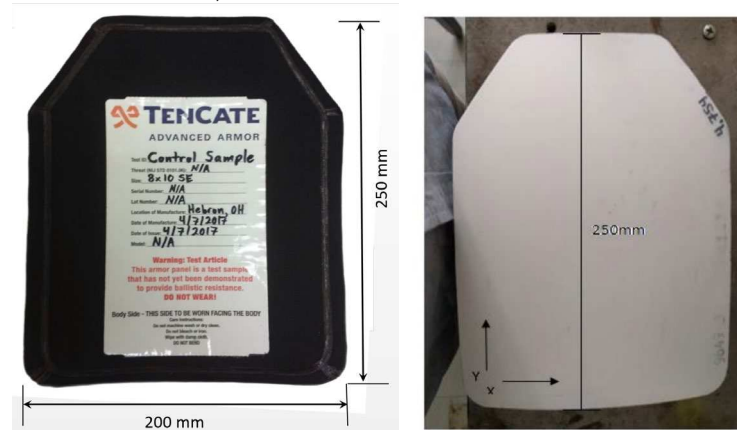
Figure 1. Geometry of control plate donated by TenCate, Integris Composites Inc. (a) Armor plate with cover. (b) Defective plate with outer fabric removed.
