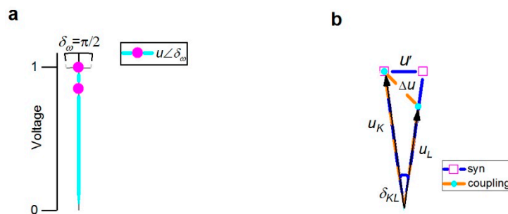
Figure 1. Schematic diagram of the power system operating coordinate system (U, \delta_\omega) .
