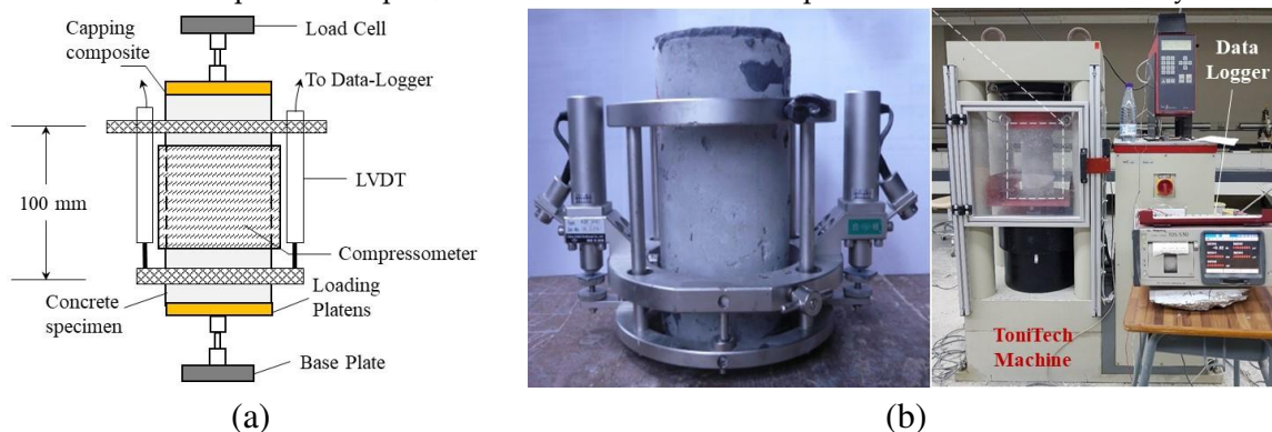
Figure 9. The uniaxial compression test: (a) representatives' diagram and (b) detailed setup.
