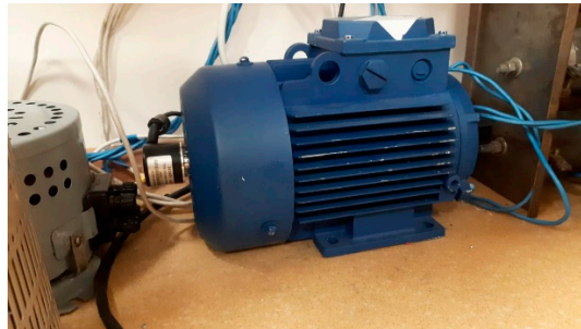
Figure 79. The load of the regulator.
