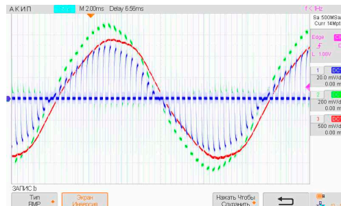
Figure 74. The shape of the input and output voltage with current (green U_{out} , blue I_{out} ).
