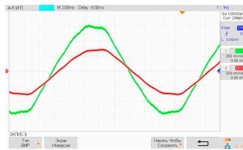
Figure 75. Voltage waveforms of capacitors (red U_{in} , green U_c ).
