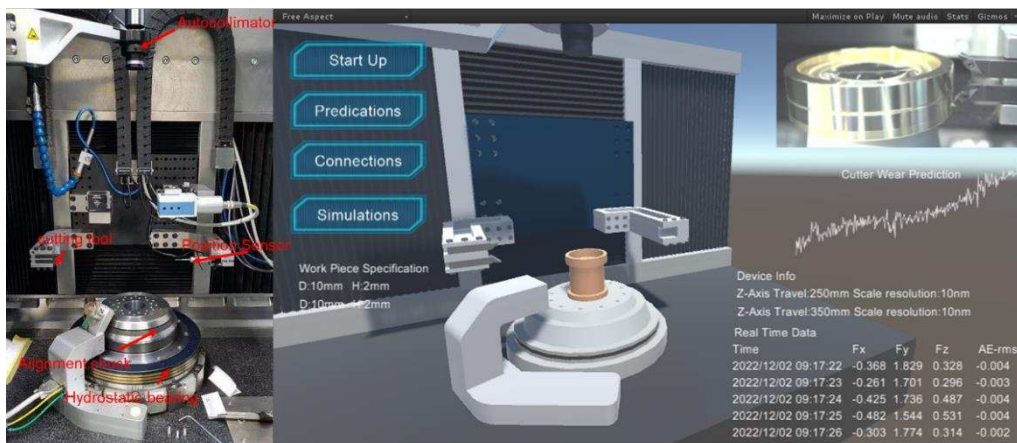
Figure 10. The main interface of the digital twin system for the high-precision lens-centring process
