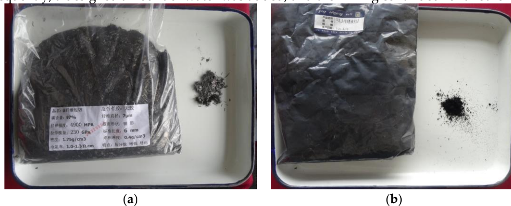
Figure 5. The CNM materials: (a) the chopped carbon fibre sourced from Toray Industries, Inc.; and (b) the nano-carbon black sourced from Suqian Xigu Nanotechnology Co., Ltd.
