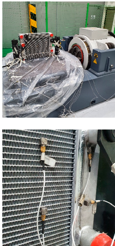
Figure 3. Experimental setup: radiator equipped with acceleration sensors mounted on a vibration dynamo.
