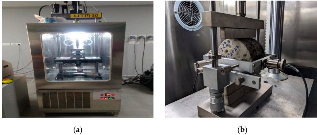
Figure 4. (a) Servo hydraulic cyclic test equipment: (b) Cyclic Indirect Tensile Test Arrangement.
