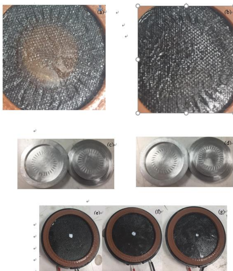
Figure 5. Photographs for fabricated nanocomposite diaphragm drivers and headphones (a) driver GOPC-L, (b) driver GOPC-C, (c) line patterned molds, (d) curve patterned molds, and (e) headphone GOPC-T1-WF3, (f) headphone GOPC-T2-WF3, (g) headphone GOPC-T3-WF3.
