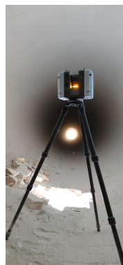
Figure 4. Leica RTC360 inside rotary kiln
