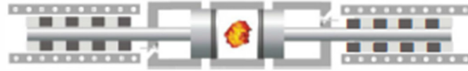
Figure 5. Schematic diagram of a linear combustion engine with a central combustion chamber and integrated gas springs [36].
