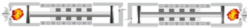
Figure 2. The basic principle of two separate units of a linear combustion engine with one combustion chamber and a gas spring [36].
