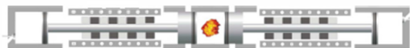
Figure 4. The basic principle of the arrangement of a linear combustion engine with a central combustion chamber in the middle [36].
