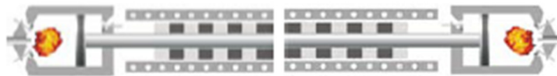
Figure 6. Scheme of the principle arrangement of a linear combustion engine with combustion chambers on opposite sides [36].
