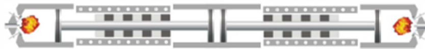
Figure 3. The basic principle of arranging two separate pistons in a cylinder with a common gas spring in the middle [36].
