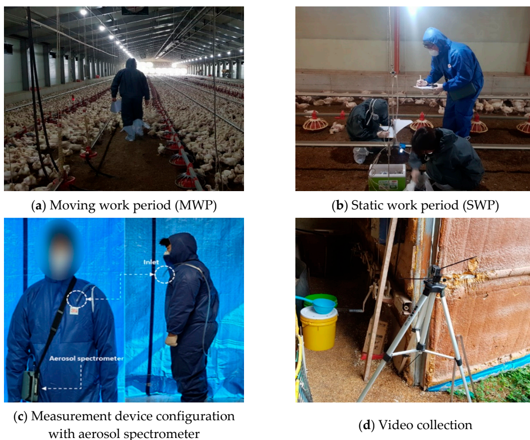
Figure 4. Real-time monitoring of working environment through working route analysis and aerosol spectrometer measurements.
