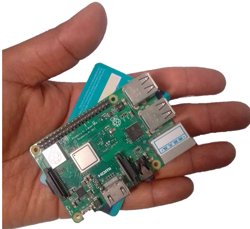
Figure 1. Sizing of a RPi compared with a credit card.
