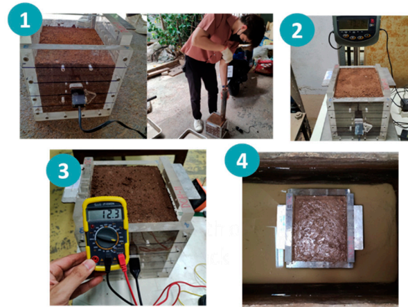
Figure 3. Calibration process for soil moisture sensor: (1) sample preparation, (2) sample weighing, (3) Sensor reading at different compaction moisture contents and (4) Final soaking.
