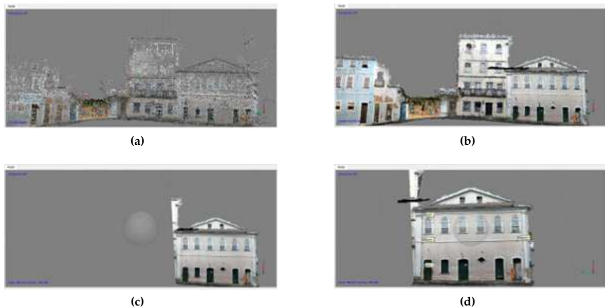
Figure 4. (a) Sparse cloud, (b) Dense cloud, (c) Mesh, and (d) Orthophoto.
