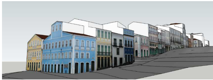
Figure 8. Integration step of the historical buildings' models with the digital terrain model.
