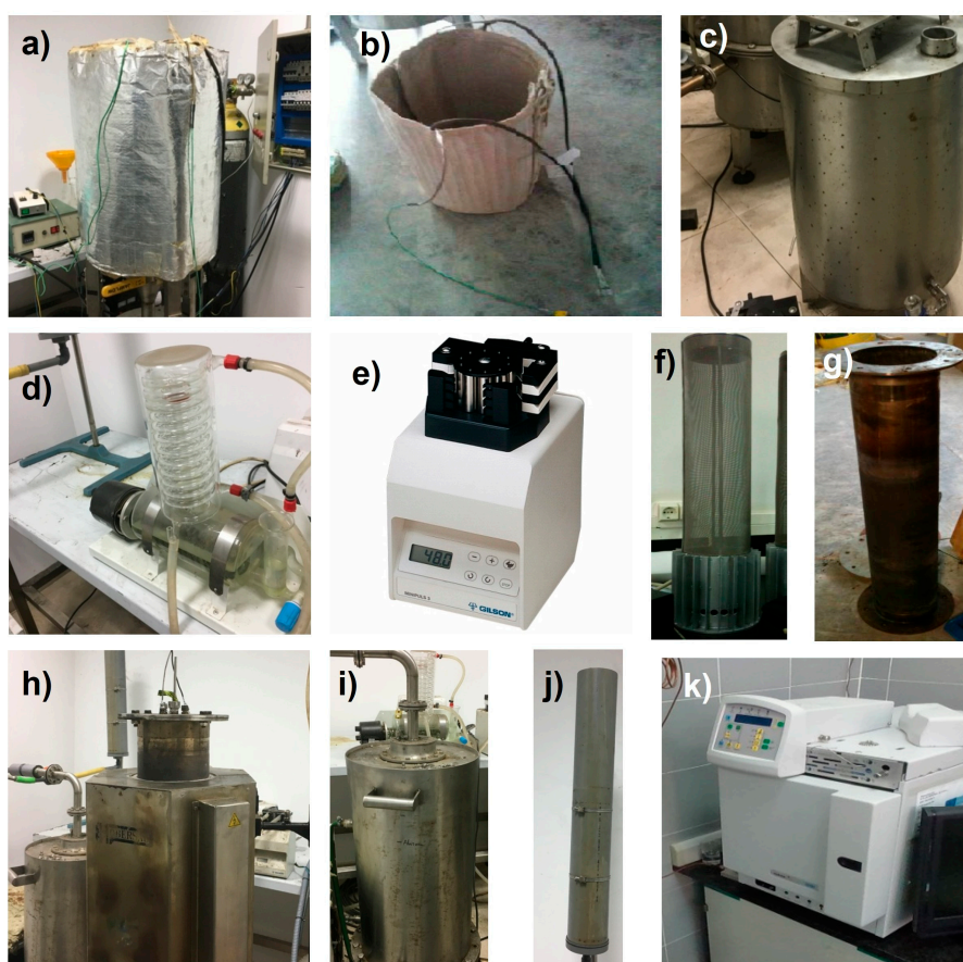
Figure 5. Different components in glycerol steam reforming system: a) drying system; b) heating jacket; c) glycerol-water mixture tank; d) distiller; e) peristaltic pump; f) basket; g) reactor; h) oven; i) heat exchanger; j) flow-meter; k) gas chromatograph.
