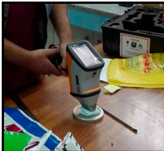
Figure 3. Analysis of plastic bag using HH XRF.
