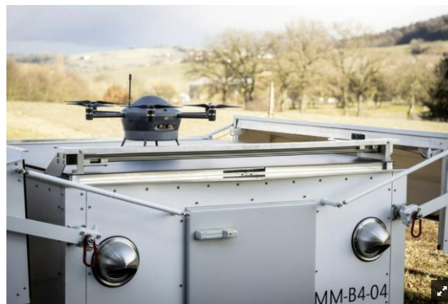
Figure 1. Meteodrone and Meteobase installed at Payerne.
