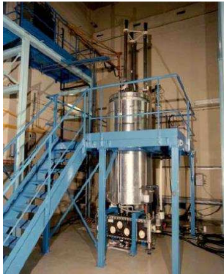
Figure 2. Experimental device of the PU+ program. Reflector vessel with instrumentation above.
