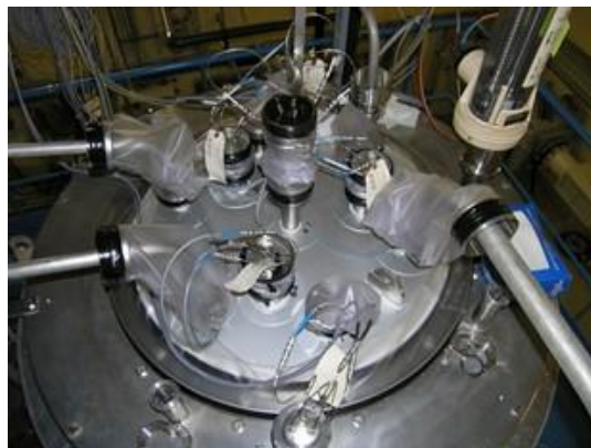
Figure 6. Overview of the solution tank with instrumentation.
