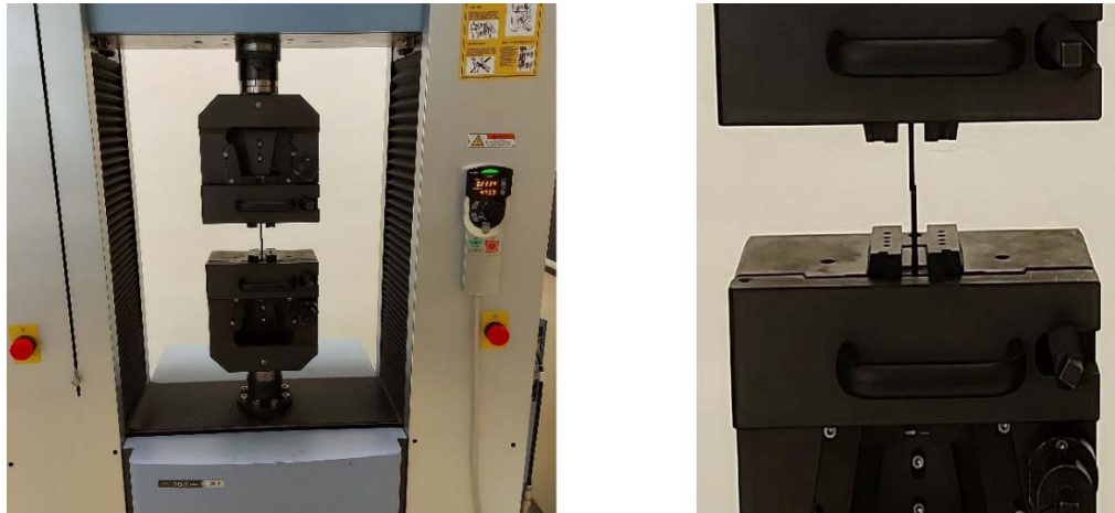
Figure 7. Experimental equipment: (a) SHIMADZU AG-X; (b) performing quasi-static uniaxial tensile stress on the test specimen.
