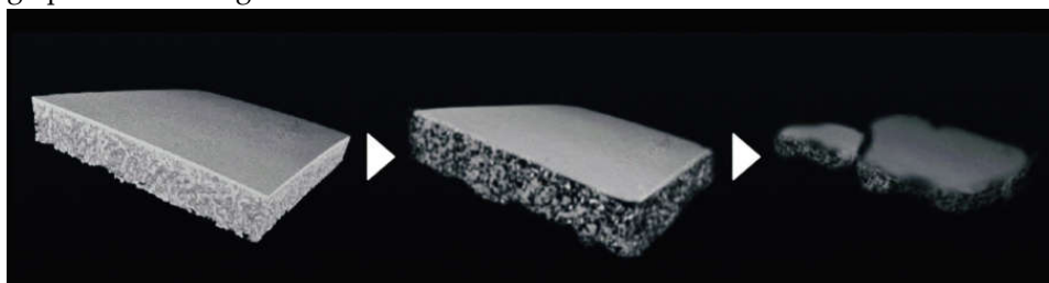
Figure 5. Schematic images of PLACL degradation provided by GC, Tokyo, Japan.
