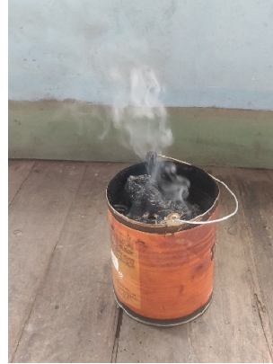
Figure 13. Smoke Recorder for Determining Wind Direction in the Main Hall. Note. Source: Author.
