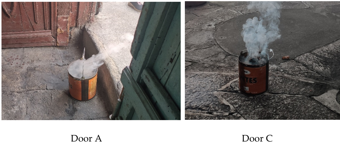
Figure 10. Smoke Recorder for Determining Wind Direction During the Afternoon. Note: Source: Author.
